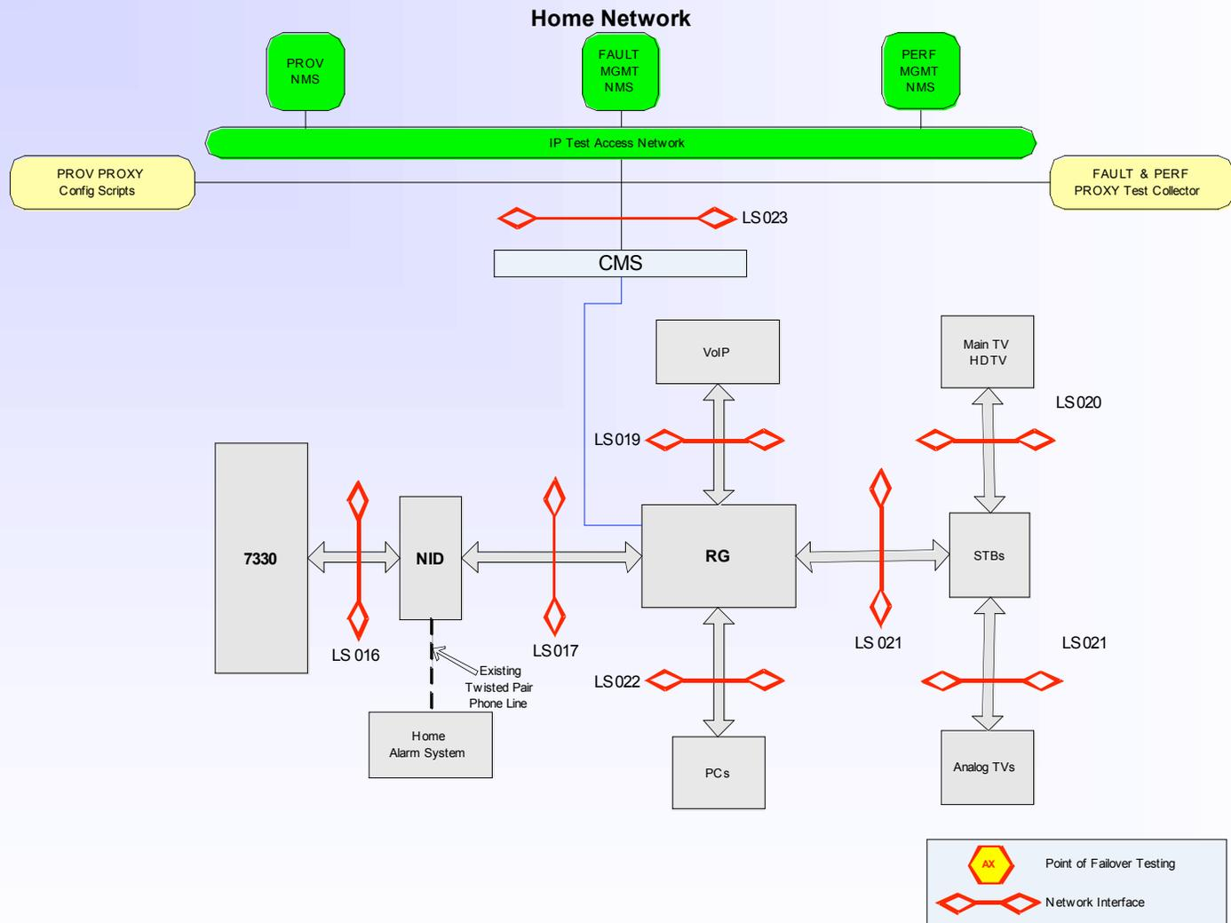
The Home Alarm System could be connected to either traditional POTS line , or a VoIP connection , pending VoIP's approval by the alarm companies .
